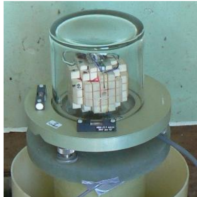
Figure 4: The IPGP VM391 tri-axis fluxgate magnetometer.
